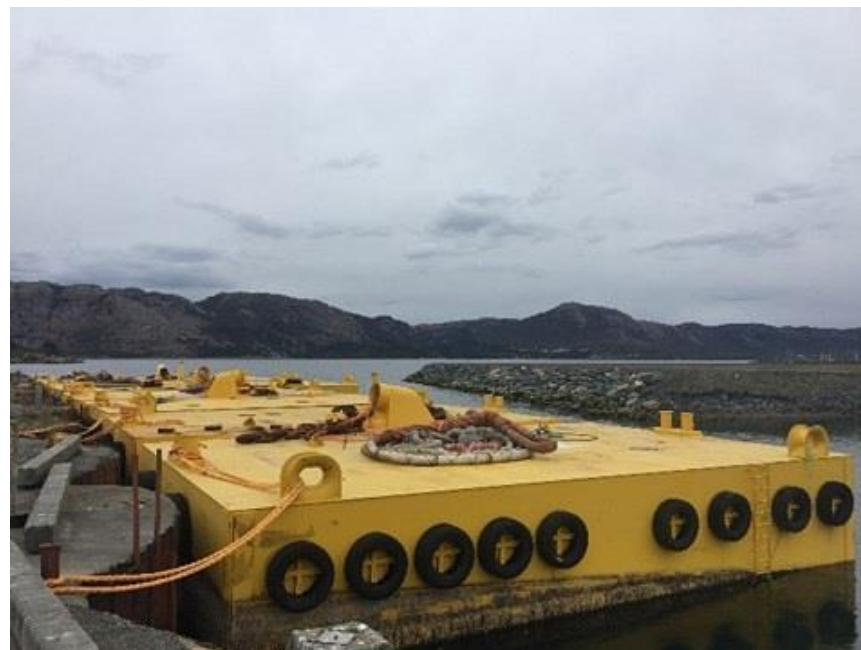
Tension Barge 14,5 x 20 x 3 meter.
