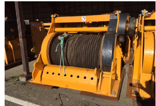
15 Ton electric pulling winch, 100 Ton holding
