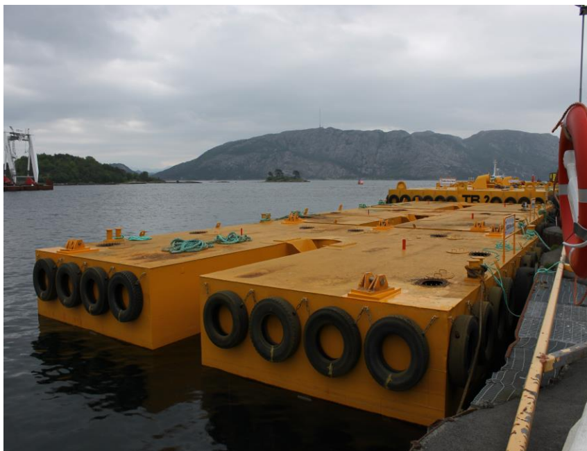
Anchor Pontoon barge 12 x 12 x 2 meter.
