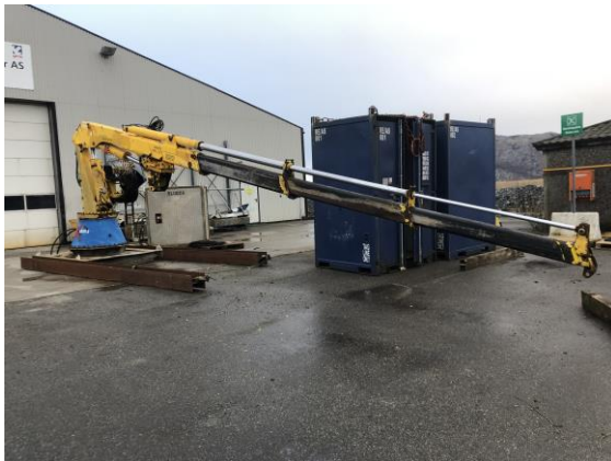
Folding crane 2.1 ton @ 10.87 mtrs
