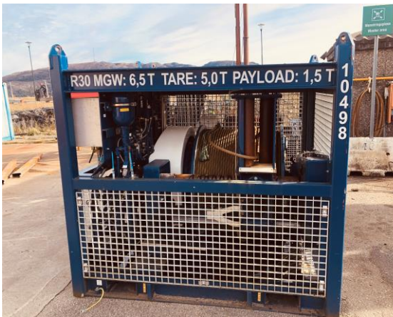
5 Ton hydraulic Constant Tension zone 2 winch Spooling system, high speed and radio control
