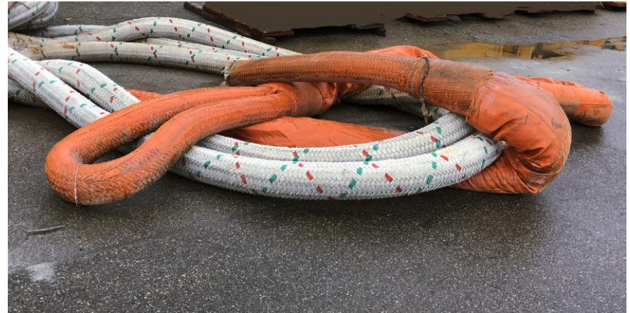
205 mm fiber rope, 44 meter length, soft eyes, MBL 1240 Ton
