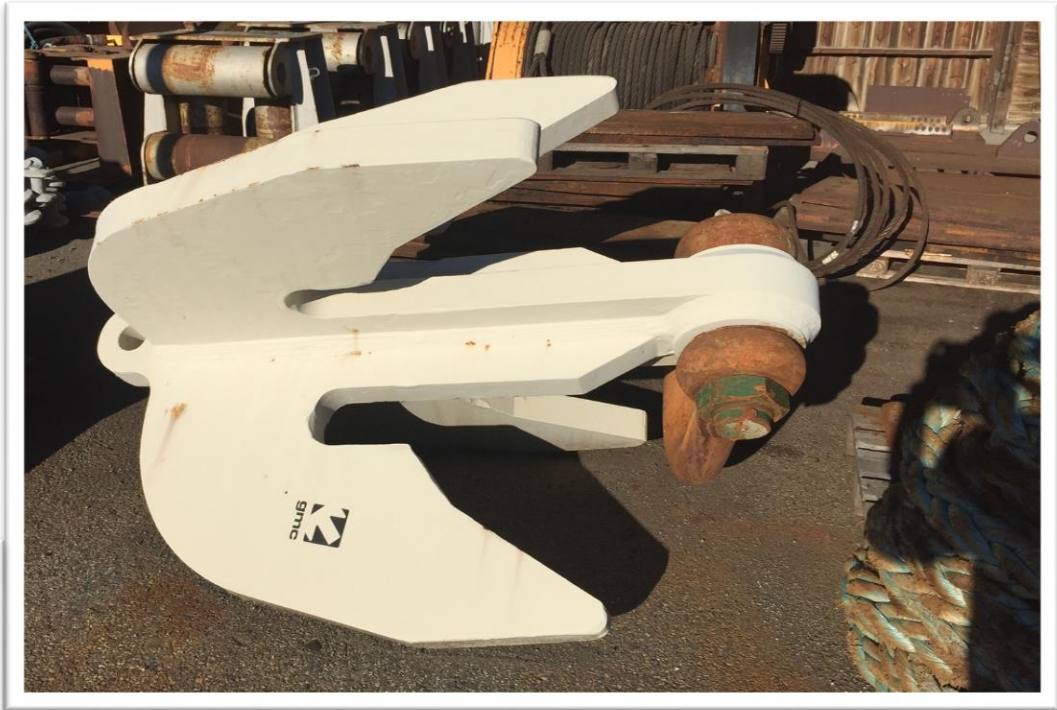
BEL 139 Grapnel, capacity 250 Ton, tested to 350 Ton
