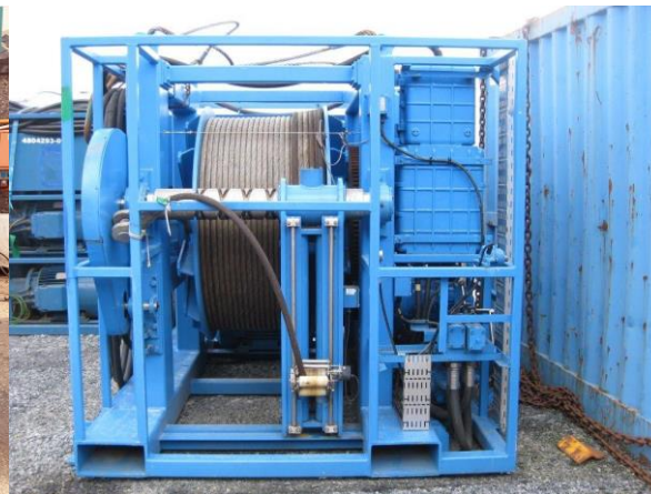
14 Ton electric Constant Tension zone 2 Spooling system and high speed
