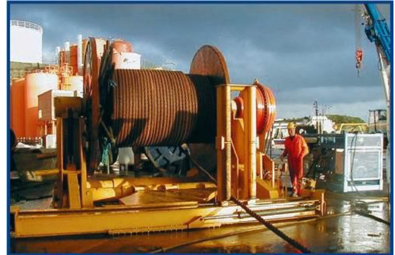
150 Ton capacity spooling machine Tension readout and level wind spooling system. Max drum diameter 6.2m, max drum width 8m 30T back tension. Comes with diesel HPU.
