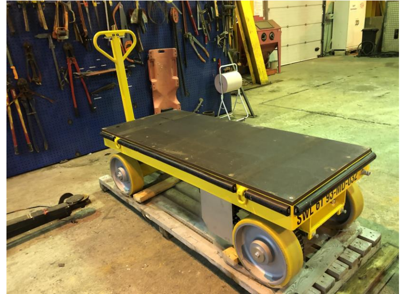
Air 6 Ton transport trailer Padeyes for lifting empty trailer and strapping. One-wheel drive and front wheels turning
