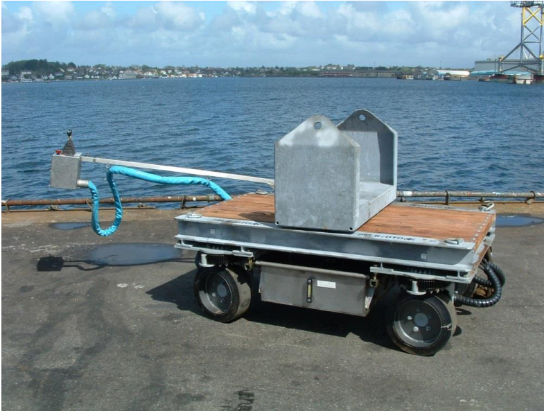
Air-hydraulic 6 Ton transport trailer Padeyes for lifting empty trailer and strapping. Four-wheel drive and four wheel 350 deg turning.
