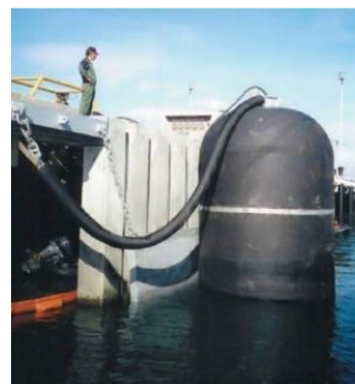
Yokohama air fender in vertical position
