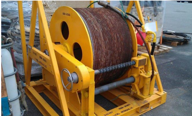
5 Ton hydraulic high speed lifting winch
