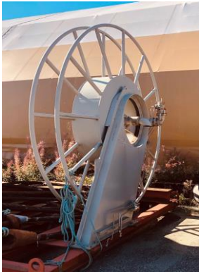
Hose or rope storage winch
