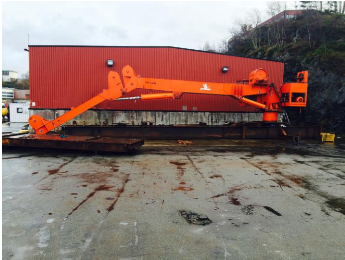
Offshore deck crane 5 T @ 20 mtrs
