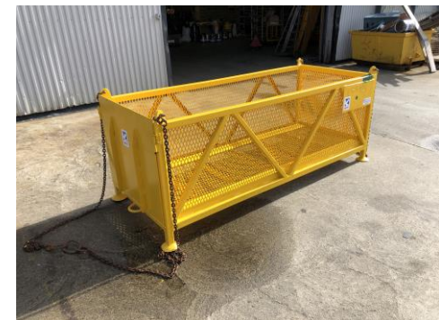
Subsea equipment baskets
