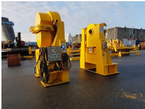
125 Ton capacity spooling machine. Max drum diameter 6m, max drum width 5 m 5 Ton back tension. Comes with diesel or electric HPU.
