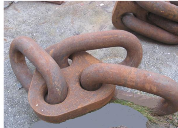
300 Ton capacity Tri-plate with links
