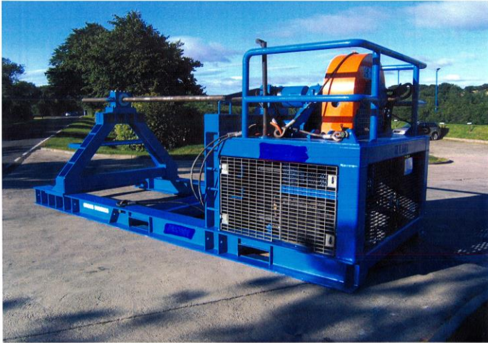
125 Ton capacity spooling machine. Max drum diameter 6m, max drum width 5 m 5 Ton back tension. Comes with diesel or electric HPU.
