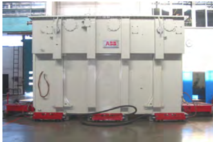
Thanks to the air bearing elements, the load can be easily lifted from the floor.
